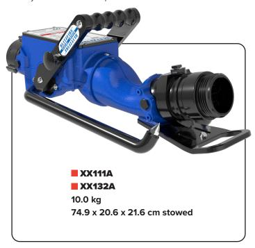
slide valve. The discharge pivots make directing the stream extremely quick and effortless. Outlet has built-in stream shaper. A unique up/down pivot on the hose inlet allows the monitor to have stability even on porches and stair landings. Folding legs have replaceable carbide tipped spikes. An anchor strap is included for safe operation.
