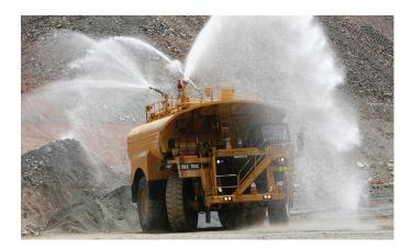
TFT's TORNADO RC compact industrial monitor is designed for both fire and industrial applications. This industrial version is certified to ingress protection IP66/67 to limit penetration of dust and moisture into the electronics, ball races and gears. Models are remotely operated and are capable of flowing up to 2000 l/min. Heavy duty seals and O-rings help mitigate contamination in applications like mining and road construction.
