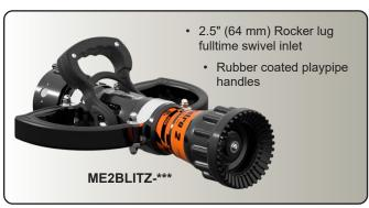
Flow calibration is specified at order entry per the ordering matrix. The specified flow calibration disc will be installed at the factory; the nozzle will NOT be sent with extra flow calibration discs. To change flow calibration, a flow disc kit is required. Each kit includes a set of flow washers, retaining rings, instructions and the service tool. See page T2 for kit ordering information.
