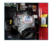
TFT offers a BIV solution for every application. Options include handle placement, inlet/outlet sizes, body profile, pressure relief, and remote control. Design your BIV to fit your unique apparatus.
