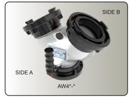
To change a 4" (102 mm) or 5" (127 mm) Storz from rigid to full-time swivel, back out the lockout screw until the coupling moves freely. See page T4 for diagram.
