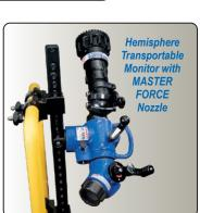
The Master Force nozzle is equipped with a low pressure override knob which allows the nozzle to achieve greater flows at lower pressures. The operator simply selects either the standard 100 psi (7 bar) or 55 psi (4 bar) setting by turning the knob at the front of the nozzle.
