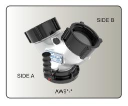
To change a 4" or 5" (102 or 127 mm) Storz from rigid to full-time swivel, back out the lockout screw until the coupling moves freely. See page T4 for diagram. All 6" Storz couplings have an adjustable seal compression feature.
