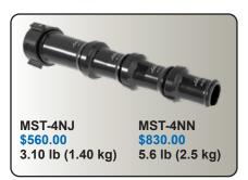
**MST-4NJ** - 4 STACKED TIPS, 2.5" NH (64 mm) Designed for monitor use, these lightweight tips are hardcoat anodized, allow four orifice options in one, and have pressure/flow charts laser engraved on each tip. 2.5" NH (64 mm) swivel coupling is standard. Orifice openings are 2", 1.75", 1.5", and 1.375". (51 mm, 44 mm, 38 mm and 35 mm) Length 16.90" (42.9 cm)
