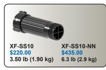
**XF-SS10** - STREAM STRAIGHTENER 10" L. (254 mm) 2.5" NH (64 mm) THREADS - Extruded aluminum vanes straighten smoothbore streams to provide greater reach with less turbulence. 2.5" NH (64 mm) rigid female inlet and male outlet threads are standard.
