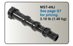
4 STACKED TIPS, 2.5" NH (64 mm) Designed for monitor use, these lightweight tips are hardcoat anodized, allow four orifice options in one, and have pressure/flow charts laser engraved on each tip. 2.5" NH (64 mm) swivel coupling is standard. Orifice openings are 2", 1.75", 1.5", and 1.375". (51 mm, 44 mm, 38 mm and 35 mm) Length 16.90". (42.9 cm)
