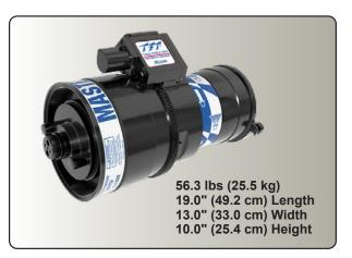
The Master Stream 4000 ER series is a super-high volume nozzle capable of flowing up to 4,000 gpm (15,000 l/min). The automatic version flows 600-4,000 gpm (2,300-15,000 l/min) and incorporates field adjustable nozzle pressure regulation capable of constant nozzle pressures from 80-120 psi (5.5-8.3 bar).
