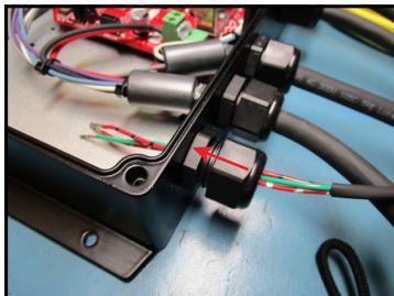
4. Feed the crimped ends of the cable through the strain relief fitting.
