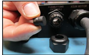
3. Remove the strain relief cap and push the rubber plug out of the fitting from the back side.
