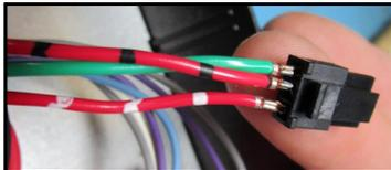
5. Push the crimped ends of the wires into the connector in the positions shown. Push the pins until they click into place.
