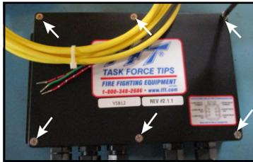
1. Loosen 6 screws on the top of the Control Box to remove the lid.
