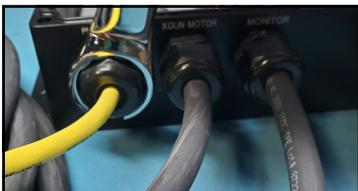
7. Position the cable in the fitting so the yellow cable jacket is just visible inside the box. Tighten the strain relief fitting until snug.
