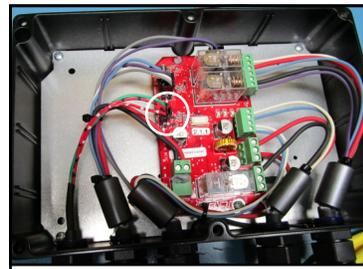
6. Plug the connector into the board header labeled "buttons". Push the connector until it clicks into place.
