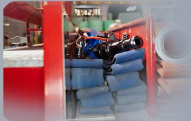
Preconnected BLITZTAC allows quick deployment
