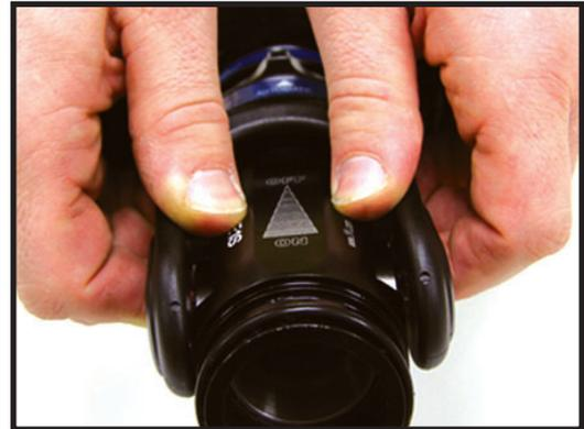
**Step 6)** Use your finger to pull out the stainless steel slide valve. Two or three o-rings seal the slide valve, there will be some resistance when it is pulled out.
