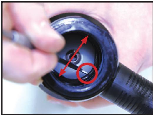
**Step 9)** Using the 3/16" Allen wrench, un-thread the valve plug from the valve. The green aluminum center will accept an Allen wrench.
