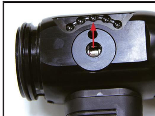
**Step 16)** Install the detent springs and balls back into the bail handle. Using the same method as when the handle was removed retain the springs and balls in the handle with your thumbs. Install the handle over the valve snapping it into place. Insure that the valve handle is oriented as indicated in the photo. The cam pin hole should be forward toward the exit of the nozzle.
