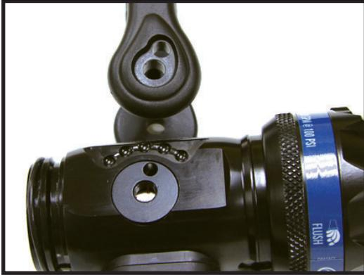
**Step 17)** Install a cam pin in each cam pin hole. Insure it seats in the groove in the slider. The cam pin face should be flush with the surrounding handle when properly installed. Apply red Loctite® to the threads of the button head screws that retain the handle. Install one on each side of the handle until hand tight.
