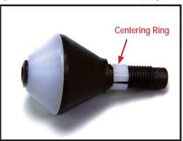
**Step 11)** Apply Blue Loctite to the valve plug. Thread the new valve plug into the valve body until snug. DO NOT tighten.
