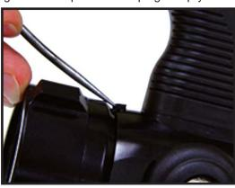
**Step 2)** Holding the nozzle over a container with the port plug hole facing down rotate the coupling until all the ball bearings fall out. 33 balls retain the coupling. Once all the ball bearings have been removed pull off the coupling, debris screen, and o-ring.
